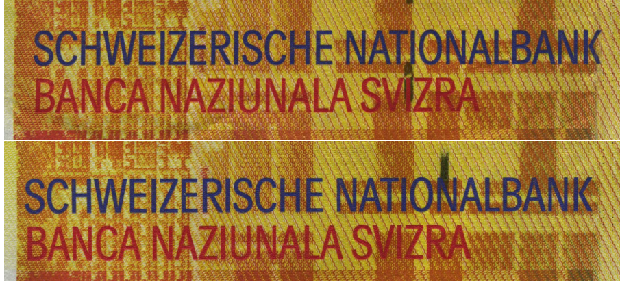
Figure 1: Comparison of two crops of different genuine CHF 10 banknotes. The text appears on different backgrounds that are not geometrically aligned.
