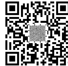
(h) Copy detection patterns and 2D bar code 1 .
